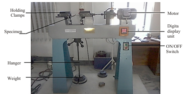
Fig. 5. Fatigue test experimental setup
